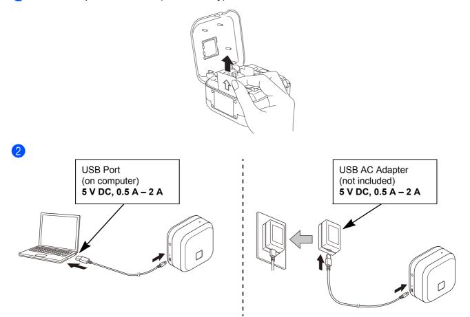
Connect the label printer to the computer using the included USB cable, or connect the USB cable to a USB AC Adapter suitable for charging mobile devices, and plug the adapter into a power source. Charge until the Battery LED turns off.
